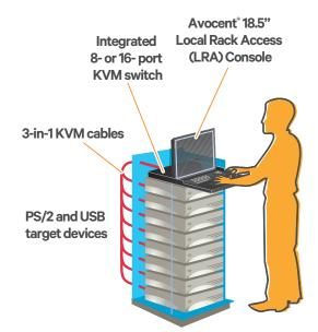
The Avocent LRA Console family provides the simplicity, efficiency and ease of use to make it the perfect in data center access point. The LRA line enables ease of access to multiple servers making software upgrades, troubleshooting and system monitoring convenient and less time-consuming.
